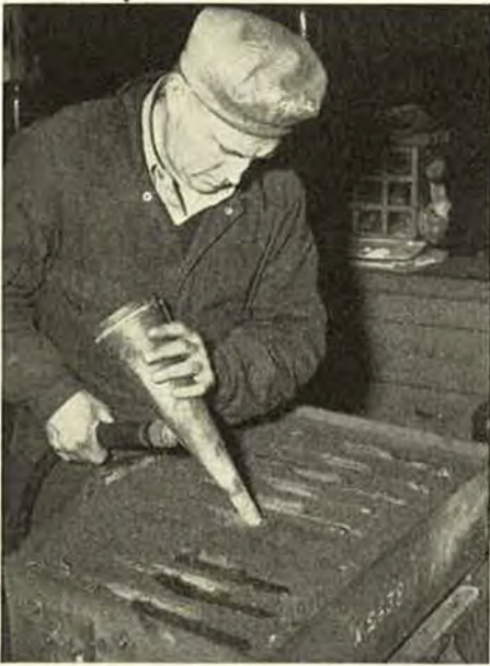
BERNIE FAULL , using the semi-automatic submerged arc welding process, reclaims tractor track assemblies by replacing metal on worn parts. This process costs only a fraction of replacing unserviceable items.
